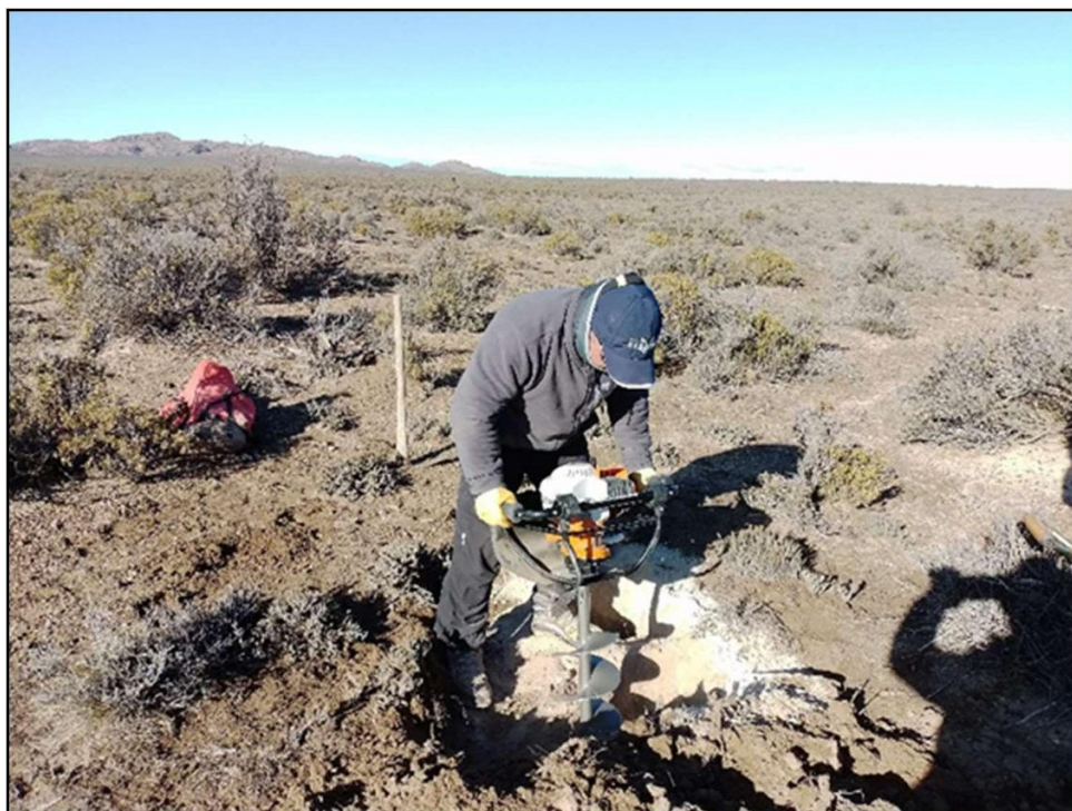
Figure 11-3. Auger drilling (excavation) of the 1.20 m by 0.90 m sampling pit area (Miller, 2024).
